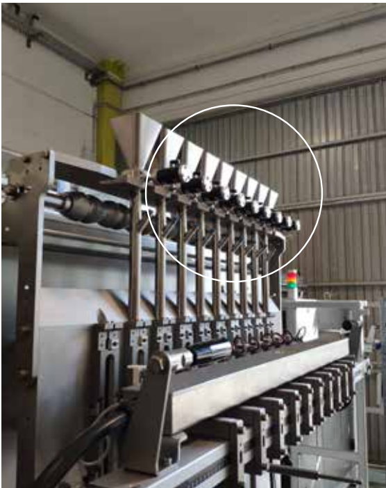
K (linear pneumatic vibrator) - Hopper emptying
