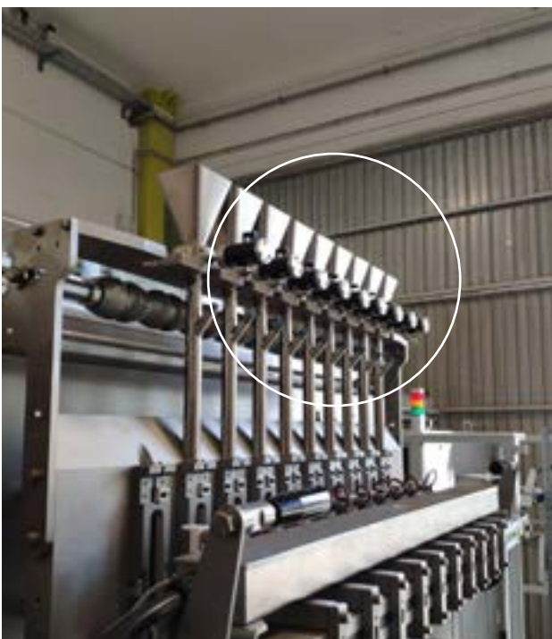
K (linear pneumatic vibrator) - Hopper emptying
